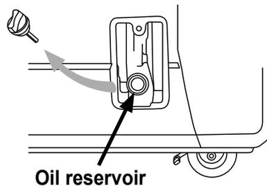
3. Check the oil level and add oil if necessary.
