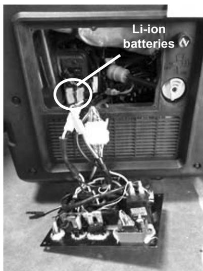
3. Remove the two Li-ion batteries.
