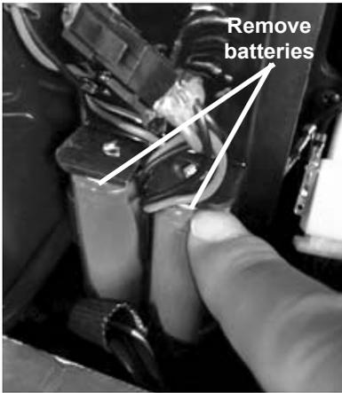
4. Insert two new Li-ion batteries.
