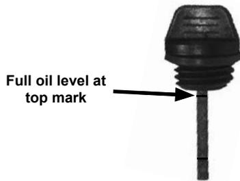
4. Reinsert and tighten the dipstick in the oil reservoir.
