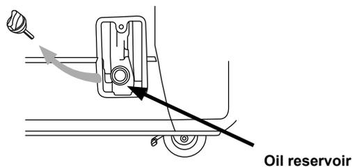
3. Insert the oil drain pipe (included with the generator) into the oil reservoir.
