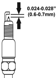
**8.** Reinstall the spark plug carefully.
