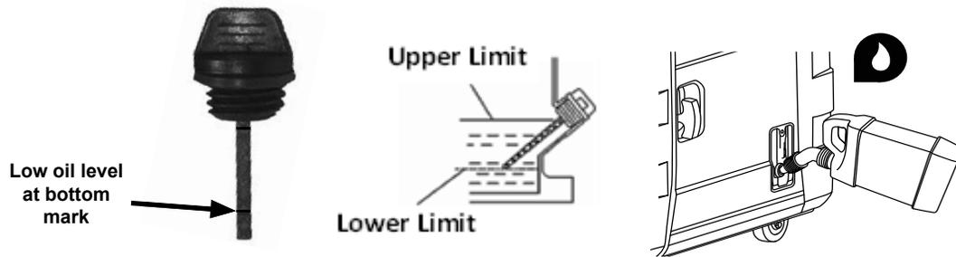
c. After refilling, check the oil level again, and ensure that the oil level is at the top mark on the dipstick.
