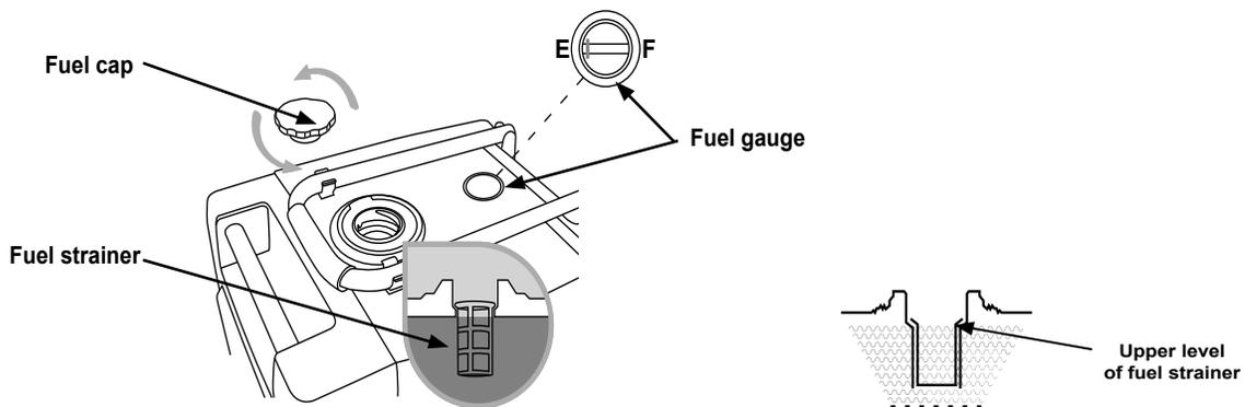
3. If fuel is low, with the fuel cap off, pour fuel slowly over the fuel strainer. Do not fill past the upper level of the fuel strainer. Avoid getting dirt, dust or water in the fuel tank.
